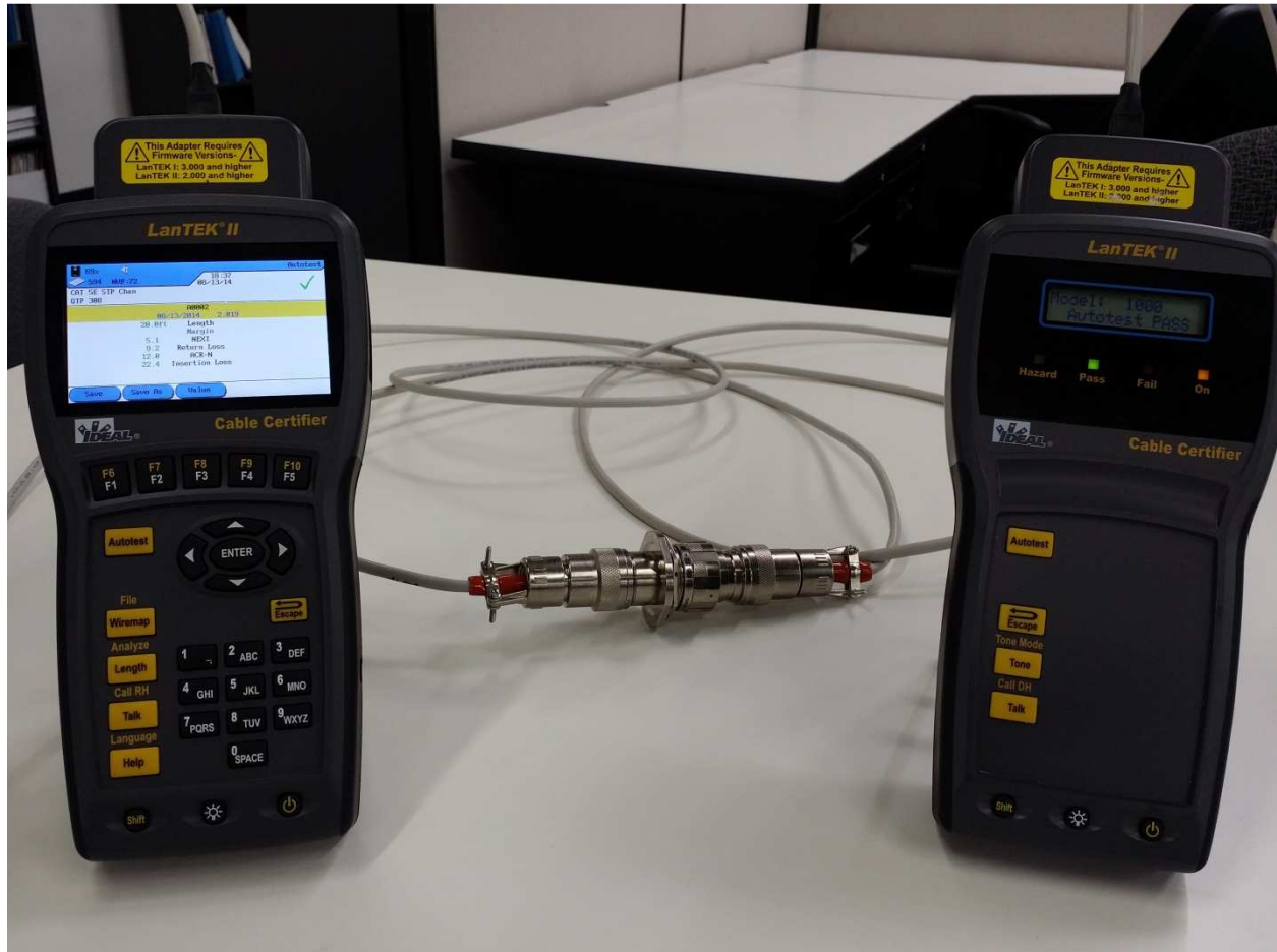
Figure 3. Ethernet Compliance Test
