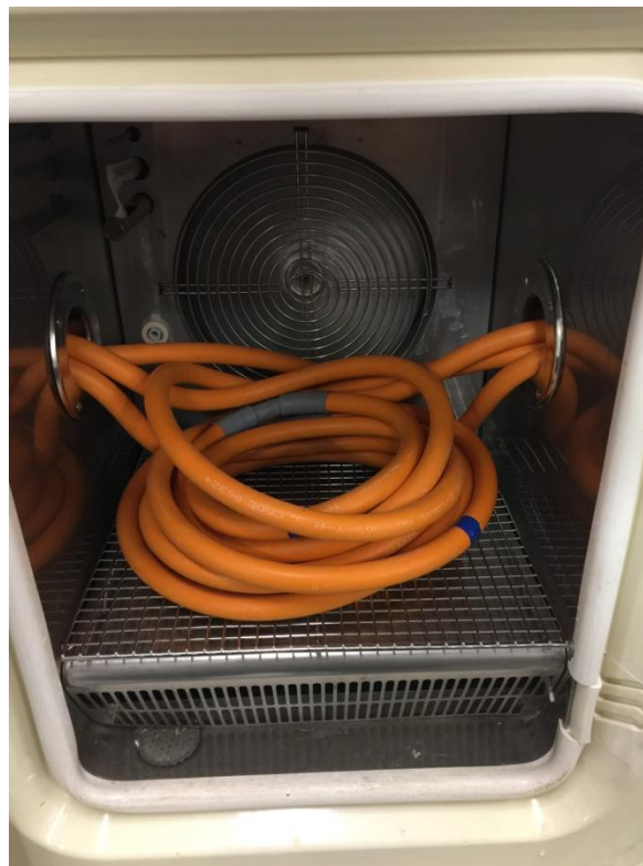
Image 6 : Curing of Autoshrink samples with adhesive. 40C @ 50% RH for 48 hours.
