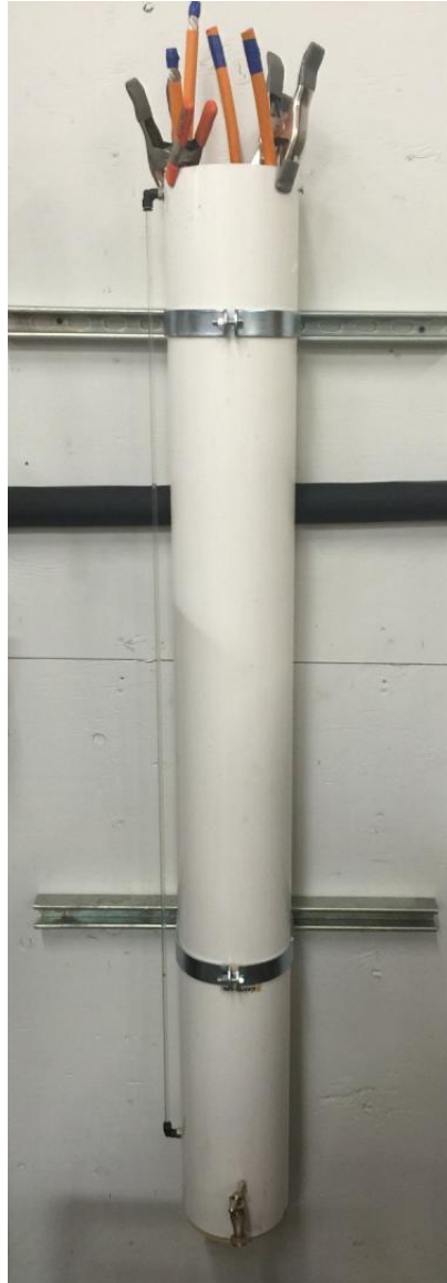
Image 2: Immersion insulation resistance tank.
