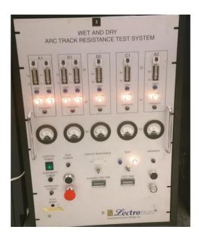
Figure 1: Lectromec wet short circuit test equipment control cabinet. Circuit C2 runs in a circuit in parallel with the control cabinet.
