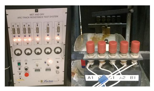
Figure 1: Lectromec wet arc track resistance test equipment control cabinet [left] and wet arc resistance test stand [right].
