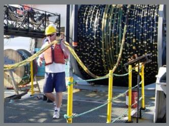
Power and data interconnects for towed-array streamers
