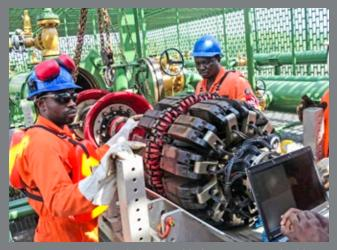
Environmentally-sealed overmolded connectors and cables for Intelligent In-Line Inspection (PIG) applications
