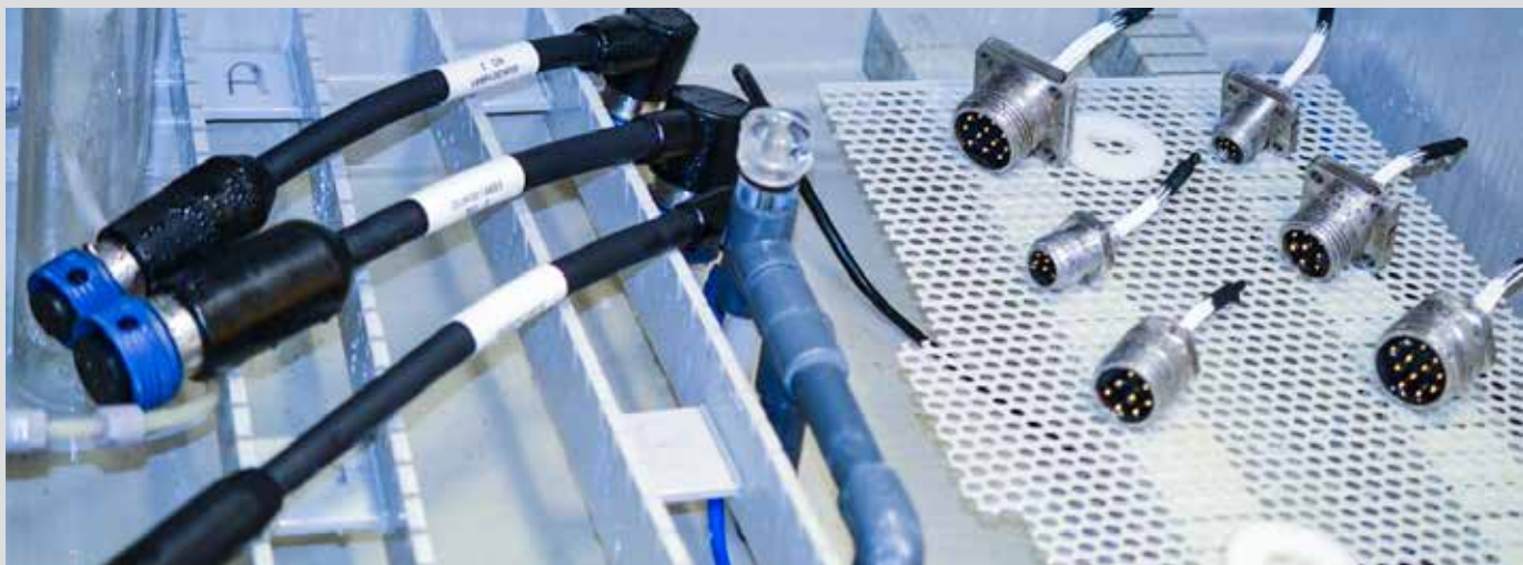
SuperG55 connector assemblies undergoing rigorous qualification testing in the salt spray chamber
