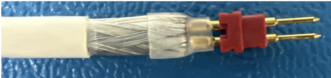
Figure 7: Shrink tube over braided shield and crimped contacts
