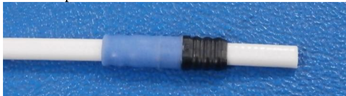
Figure 2: Clean cut cable
