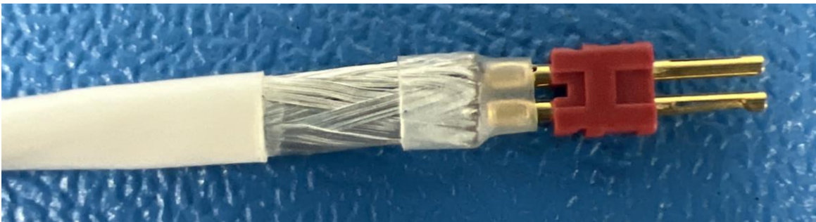
Figure 7: Shrink tube over braided shield and crimped contacts
