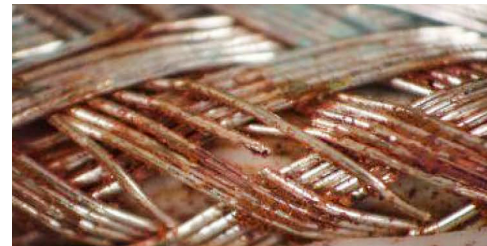
Red Plague corrosion (courtesy NASA)
